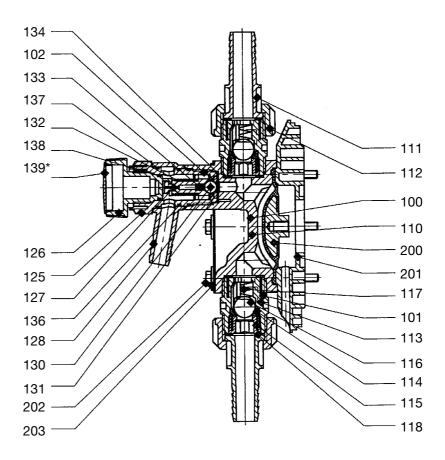
Overflow valve Sigma/ 2 liquid end, 10 bar PVT Overflow valve Sigma/ 2 liquid end, 7 bar PVT Overflow valve Sigma/ 2 liquid end, 4 bar PVT Identcode Type: 12050, 12090, 12130 Identcode Type: 07120, 07220 Identcode Type: 04350 Fig.
